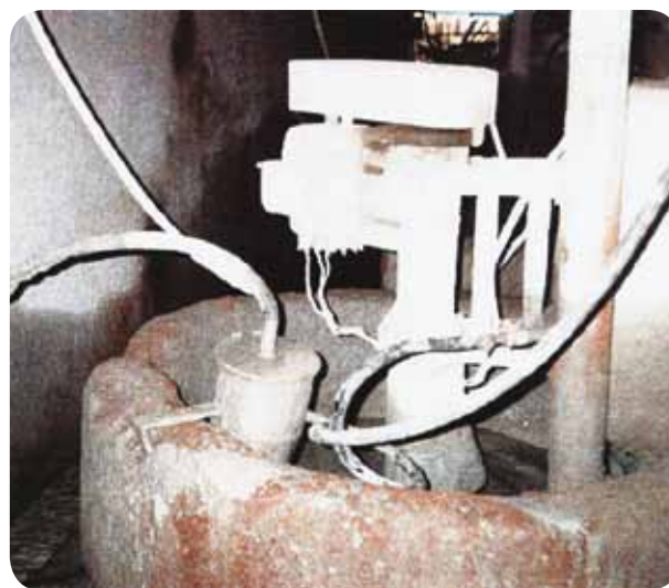
Photo 54. An abrasive sludge pumping tank; the disposal of a portion of the abrasive sludge along a collection gutter
